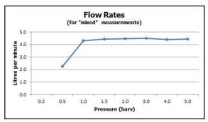
'imixed measurements' refers to equal hot and cold water supply flow rate for unregulated flow unless flow regulator fitted as standard
