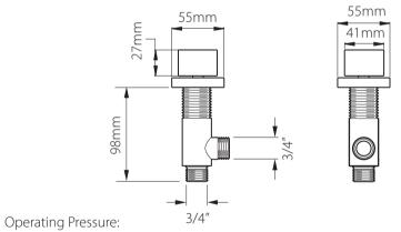
Minimum operating pressure 0.2 bar - Maximum operating pressure 5 bar
