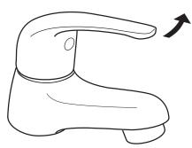
Cold tap - turning the control handle anti-clockwise will increase the flow of water.
