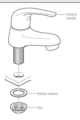
Before installing your new tap, flush through the pipework to ensure removal of debris, turn off the water supply.
