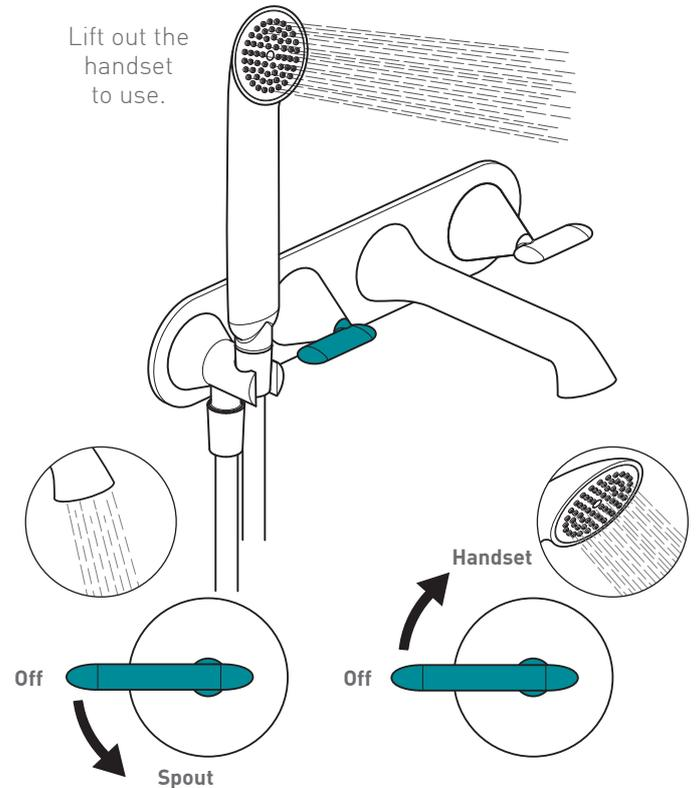
Turning the handle 90° anti-clockwise will progressively increase the flow of water to the spout (Outlet 1).
