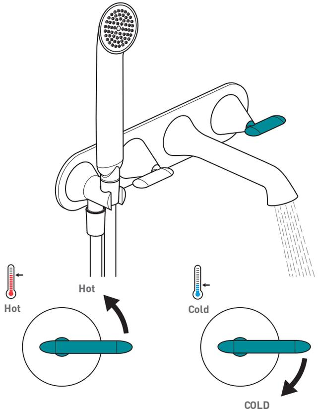
Turning the lever anti-clockwise will increase the temperature.
