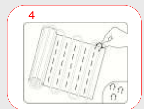
Fix the mat on to the insulation boards
