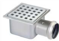
Shower Drain with Trap (Low Height) Brushed Stainless Steel 304 Grating with Anti-odour 35 mm Water Seal with Removable Trap Horizontal Outlet Dia. 40 mm Capacity - 22 l/m 105 x 105 mm Brushed Stainless Steel Code:AQD-413-LOW-BS
