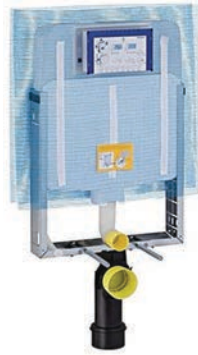
UP720 Kombifix Concealed Cistern for Wall Hung WC For Installation in Block Wall Construction Installation Height Approx. 1100 mm Thickness 80 mm Code: GEB-110-772-00-1
