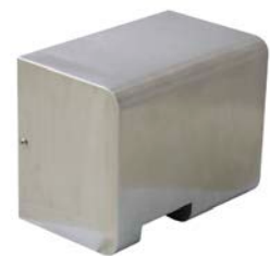
IX304 Wall Mounted Touch Free Electronic Warm Air Hand Dryer with Infrared Sensor Mains Operated Stainless Steel Grade 304 Thickness 1.0 mm 1800 Watts 220-240V, 50/60Hz IPX1 Rating 270 x 160 x 212 mm Stainless Steel Code: AQA-IX3-737-SS
