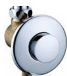
Eco-Push Self-closing Urinal Flush 3.5s Run Time Delivers 0.5L @ 4 Bar Operating Pressure Chrome Code:AQE-ECO-612200-A-CP
