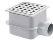
ABS Drain Brushed Stainless Steel 304 Grating with Anti-odour 50 mm Water Seal with Removable Trap Horizontal Outlet Dia. 50 mm Capacity - 25 l/m 105 x 105 mm Brushed Stainless Steel Code:AQD-615-ABS-BS
