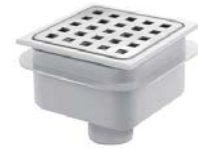
ABS Drain Brushed Stainless Steel 304 Grating with Anti-odour 35 mm Water Seal with Removable Trap Vertical Outlet Dia. 40 mm Capacity - 22 l/m 105 x 105 mm Brushed Stainless Steel Code:AQD-612-ABS-BS
