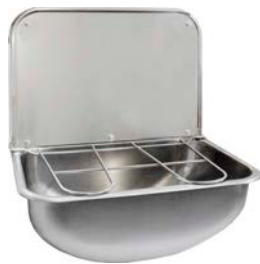
Wall Mounted Cleaners Sink Material Thickness 0.9 mm 400 x 290 x 195 mm bowl 1 1/2" Flat Perforated Waste Drainage Back Centric, 440 x 300 mm Splash Back Includes Stainless Steel Grid with Rubber Bumps and Stainless Steel Screws and Dowels Code: FRA-WB440C-SS
