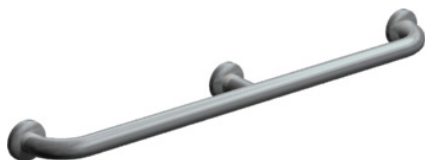
Straight Bar 32 mm O.D with 3 Support Point Horizontal or Vertical Installation 1200 mm Length Stainless Steel Code: ASI-10-3702-48-SS
