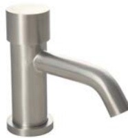
Stainless Steel Self Closing Basin Mixer with 1/2" Connection 3s Runtime Delivers 0.42L @ 4 Bar Operating Pressure Brushed Stainless Steel Code: AQM-IX3-306-SS
