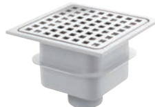
ABS Drain Brushed Stainless Steel 304 Grating with Anti-odour 35 mm Water Seal with Removable Trap Vertical Outlet Dia. 50 mm Capacity - 25 l/m 150 x 150 mm Brushed Stainless Steel Code:AQD-618-ABS-BS
