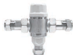
Protherm In-line Thermostatic Valve with Ceramic Cartridge 3/4" Inlet, 1/2" Outlet Supplied with 3/4" to 1/2" Adaptor Fittings Recommended for use with all Infrared Mixers Code:EBI-PRO-5001-W-NP
