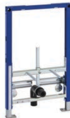
Duofix Element for Bidet for Installation in Dry Wall or Pre-Wall Construction Covered with Panel (Gypsum or Wood), for a Floor Construction of 0-200 mm Installation Height Approx. 820 mm Code: GEB-111-524-00-1
