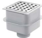
ABS Drain Brushed Stainless Steel 304 Grating with Anti-odour 50 mm Water Seal with Removable Trap Vertical Outlet Dia. 50 mm Capacity - 25 l/m 105 x 105 mm Brushed Stainless Steel Code:AQD-614-ABS-BS
