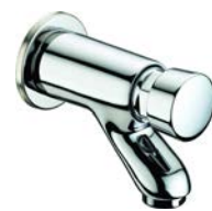
Eco-Push Wall Mounted Self-Closing Tap 14s Runtime Delivers 2L @ 4 Bar Operating Pressure Chrome Code:AQE-ECO-712109-A-CP
