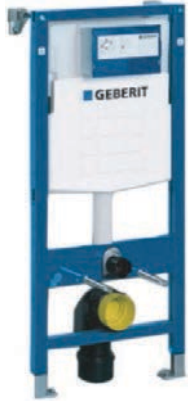
UP320 Duofix Concealed Cistern for Wall Hung WC for Installation in Dry Wall Construction Installation Height Approx. 1120 mm Thickness 120 mm Code: GEB-111-300-00-5
