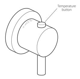
Turn the handle clockwise to decrease the temperature and anti-clockwise to increase the temperature.
