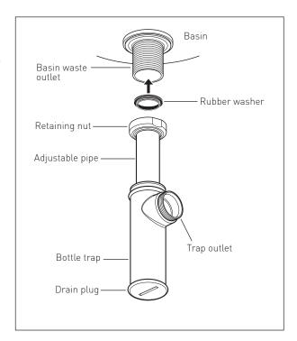
the required length. Ensure all calculations are correct before cutting, remove any burrs before assembly. Slide the retaining nut onto the overflow pipe followed by the seal, make sure that the taper on the seal is pointing towards the trap. Push the outlet pipe into the trap, slide the seal along to sit in the outlet and
