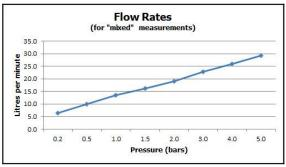
'mixed measurements' refers to equal hot and cold water supply
